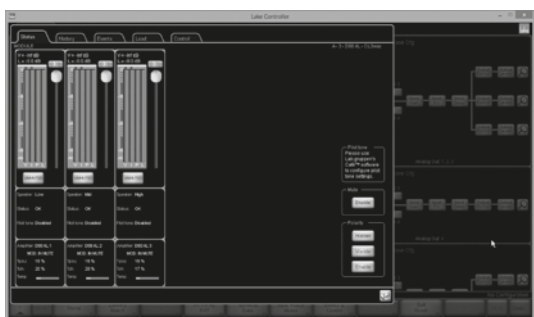
Events & Control, Status tab – Drag sliders to adjust power channel attenuation and tap mute buttons to control power channel mute. Metering and Status monitoring is available for each power channel.
